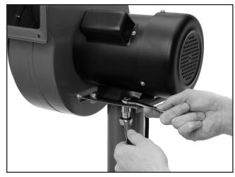
**Figure 7.** Installing motor/impeller housing on collector support.
